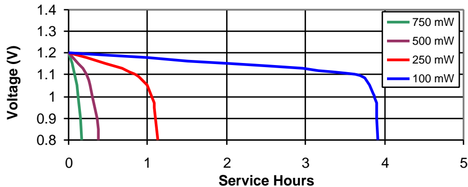
Discharge Characteristics at Various Power Drains
